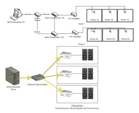
The network audio configuration of BellCommander using Barix Exstreamer or Annuncicom devices allows BellCommander to target bells and paging to zones or individual classrooms. In a zone-based configuration, a Barix Exstreamer 100 would be connected to an amplifier and speakers for each zone. In a classroom system, an Exstreamer 100 would be connected to powered speakers in each classroom.
